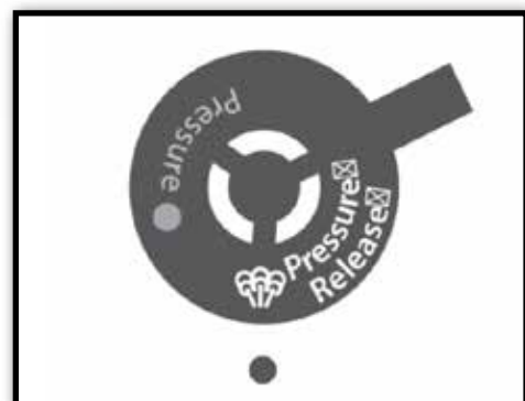
Figure 9 - Valve in “Pressure Release” position
