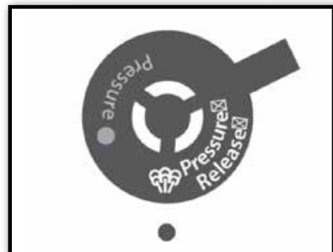
Figure 9 - Valve in “Pressure Release” position
