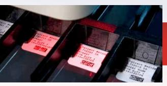
Bar code based system for reagents and samples reduces instances of user-error. Software optimized for both research and clinical settings.
